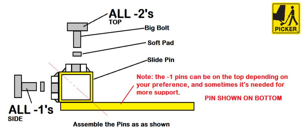
"Slide pin onto tube before this assembly starts"
